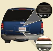
To lower the liftgate glass, push the button (figure a) under the center of the license plate lamp shield.
